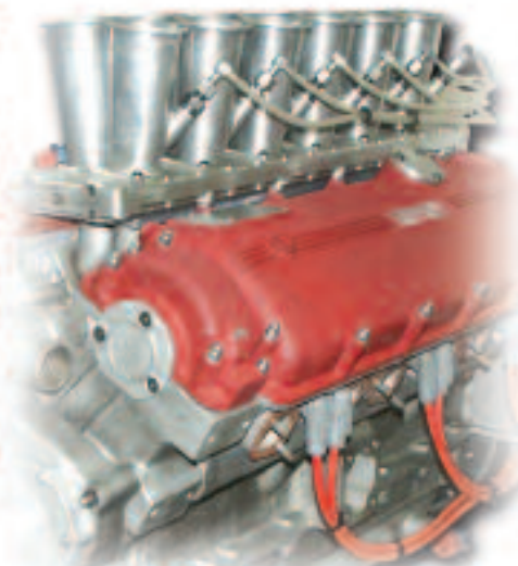
Ferrari Prototype Race Engine 450 Hp @ 7700 RPM 370 lb-ft @ 5800 RPM
